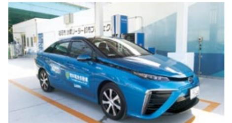
Fuel cell powered vehicle (FCV)
